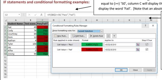
An example of an IF statement: <u>If</u> the value in column B is greater than or equal to (>=) '50', column C will display the word 'Pass'; if not then it will display the word 'Fail'. [Note that an absolute cell reference has been used]
